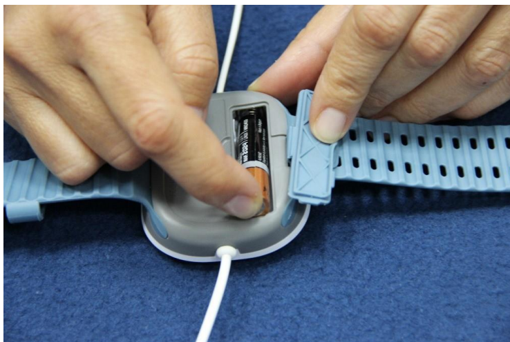
Figure 4 – Insertion de la pile
