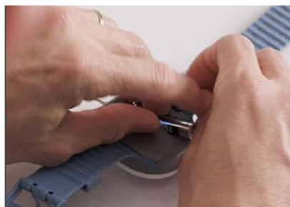
Figure 27 – Insertion de la pile
