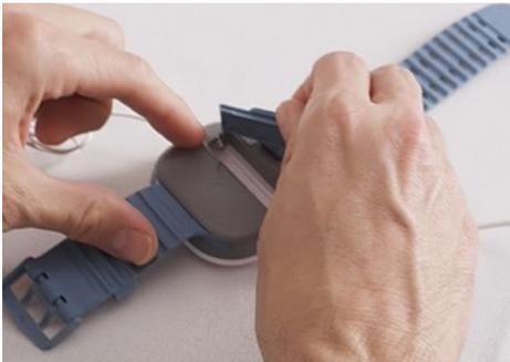
**Figure 26 – Battery removal**
