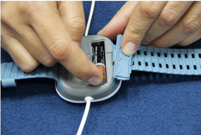
**Figure 4 – Battery insertion**
