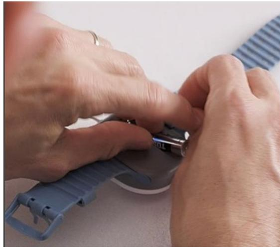
Figure 27 – **Battery insertion**
