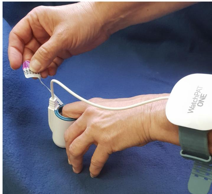
**Figure 8 – Removing TOP Tab while pressing against hard surface**
