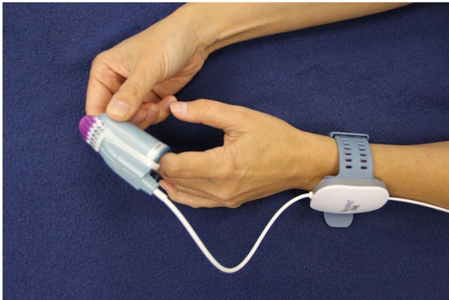
Figure 8 – Placing Finger in the Finger Probe
