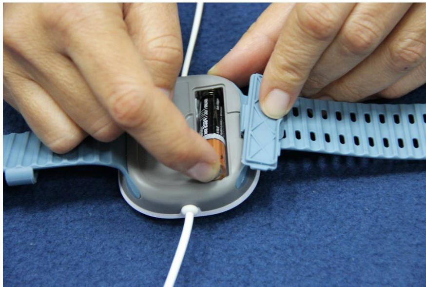
**Figure 5 – Battery insertion**
