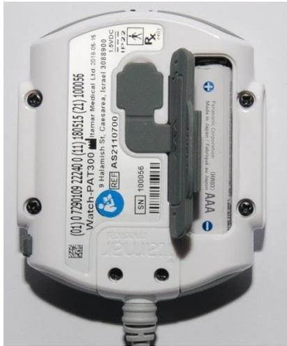
Figure 5 – Battery Compartment
