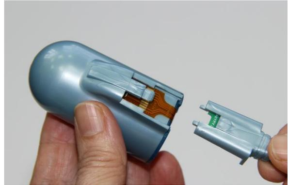
**Figure 7 – Probe Disconnected**
