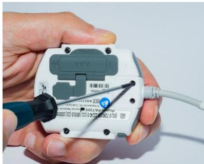
Figure 16 – uPAT Probe Cable with Screw
