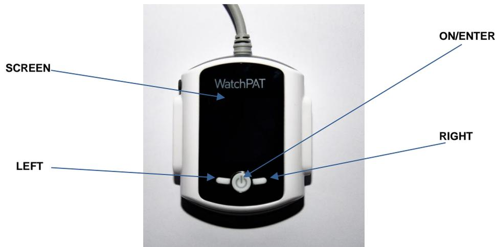
Figure 3 – The Buttons and Display
