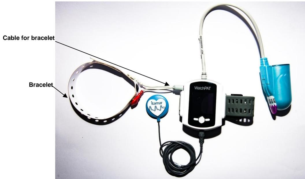
**Figure 9 – WatchPAT™ Device with Tamper-Proof Bracelet**
