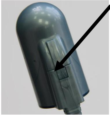
**Figure 6 – Disconnecting the Probe**
