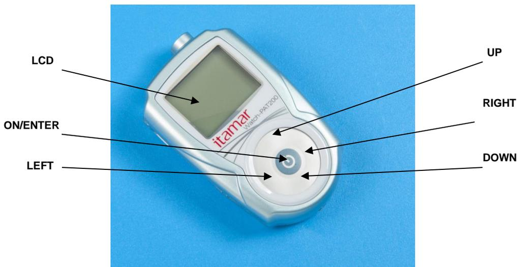
Figure 3 – The Buttons and Display
