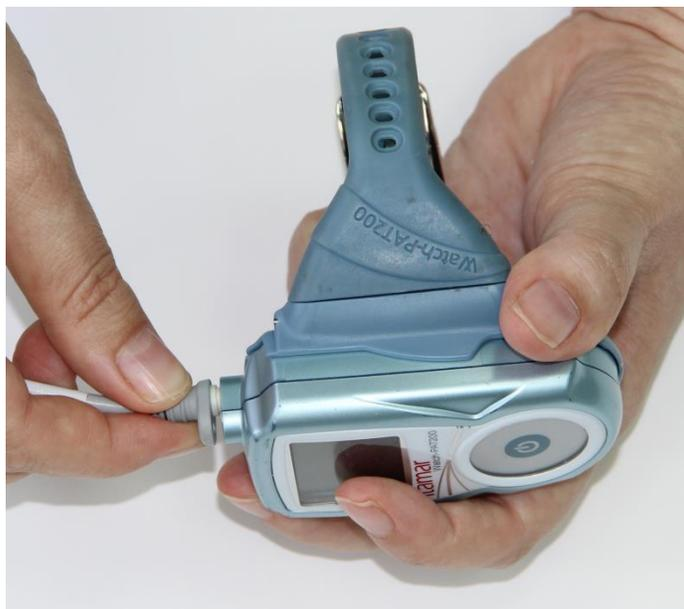
**Figure 18 – Replacing the uPAT Probe**
