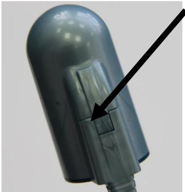
**Figure 7 – Disconnecting the Probe**
