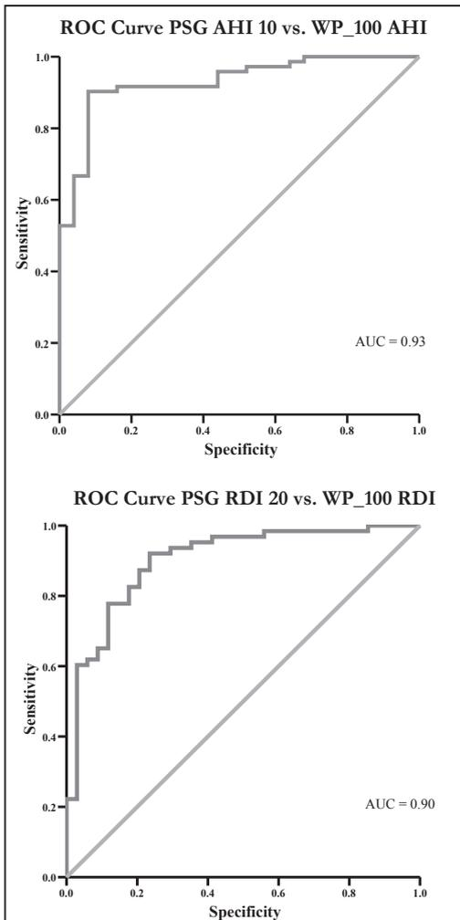
**Figure 4**—Receiver-operator characteristic (ROC) analysis shows the specificity and sensitivity for obstructive sleep apnea diagnosis of Watch\_PAT 100 (WP\_100) in this population (cut-off polysomnography [PSG] apnea-hypopnea index [AHI] >10 [a] and PSG respiratory disturbance index [RDI] > 20 [b] area under the curves [AUC] of 0.93 and 0.90,  $p < .0001$ , respectively).
