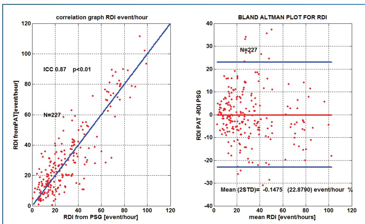
Interclass correlation and Bland Altman plot for the scoring of respiratory disturbance index (RDI). The interclass correlation between the methods was  $r = 0.87$ ,  $p < 0.01$ . On the right, the X axis represents the mean RDI between the PSG and the PAT recorder, and the Y axis the difference between methods.
