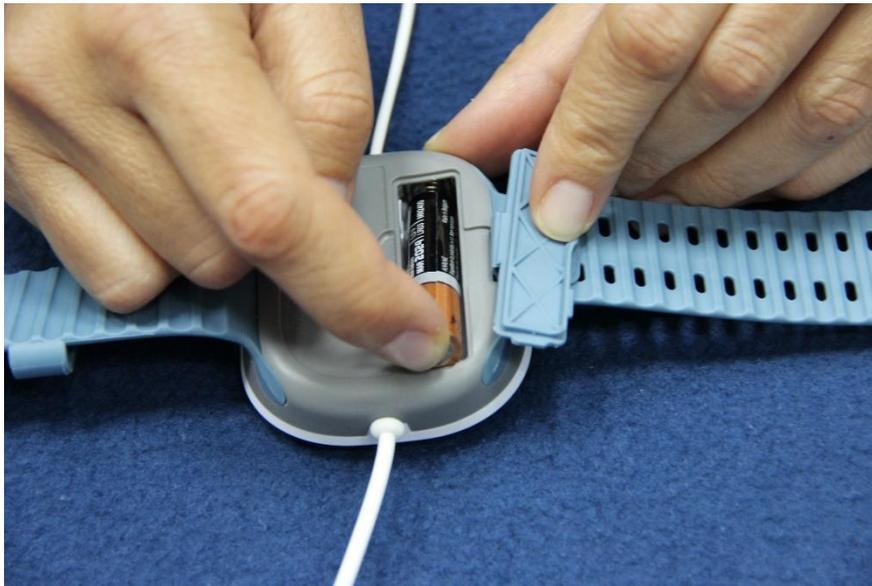
**Figure 4 – Battery insertion**
