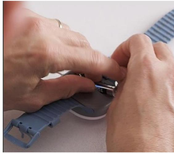
Figure 27 – **Battery insertion**
