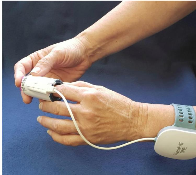
**Figure 7 – Placing Finger in the Finger Probe**
