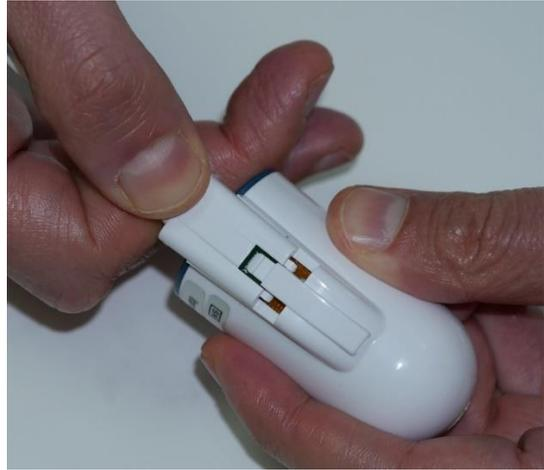
**Figure 23 – New Finger probe connection**
