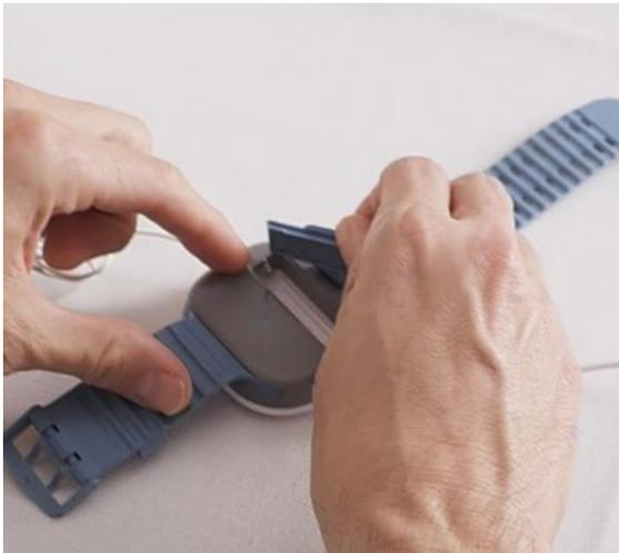
Figure 26 – **Battery removal**
