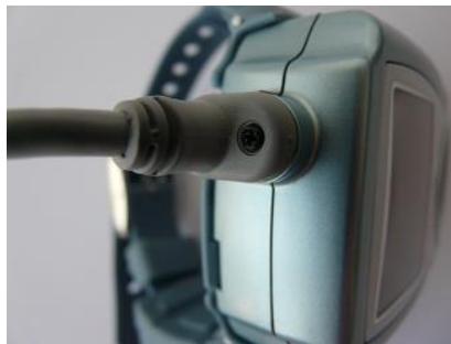
Figure 17 – uPAT Probe Cable with Screw
