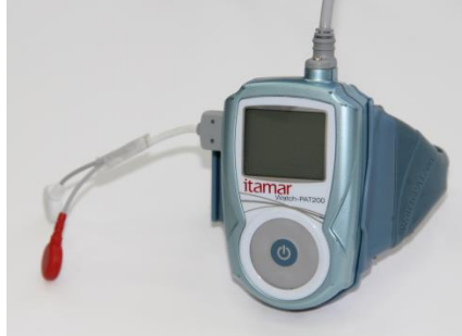
Figure 12 – WatchPAT™ Device with Cable for Bracelet
