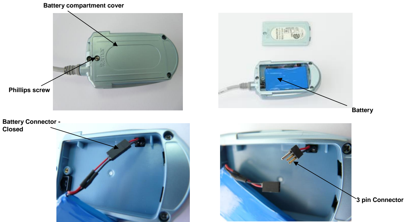
Figure 19 – Replacing the Battery
