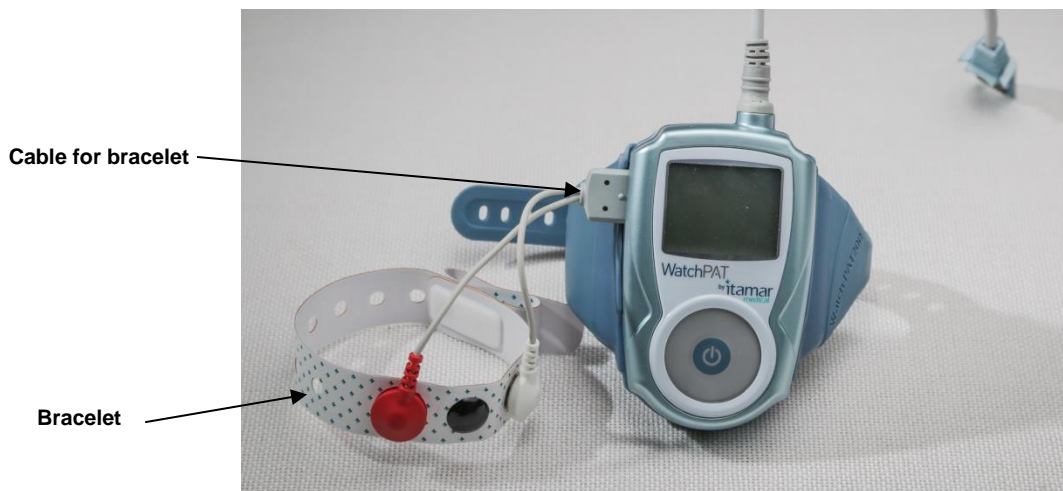
Figure 10 – WatchPAT™ Device with Tamper-Proof Bracelet
