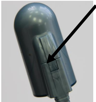
Figure 7 – Disconnecting the Probe
