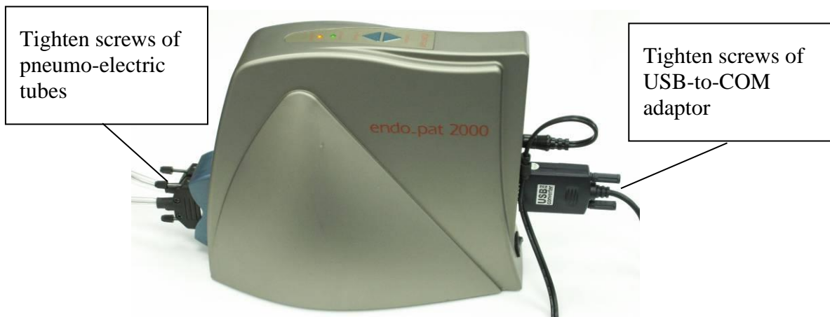
Figure 3 - Connection of pneumo-electric tubing and USB adaptor
